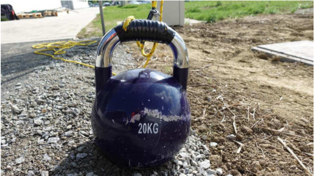
Abbildung 97: A 20 kg heavy kettlebell used for the droptests.
