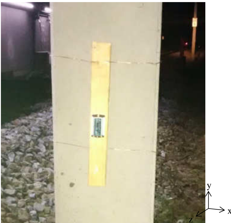
Abbildung 60: MSR-165 accelerometer mounted to the mast. The measurement axes are defined as indicated.
