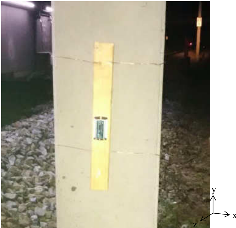
Abbildung 28: MSR-165 accelerometer mounted to the mast. The measurement axes are defined as indicated.
