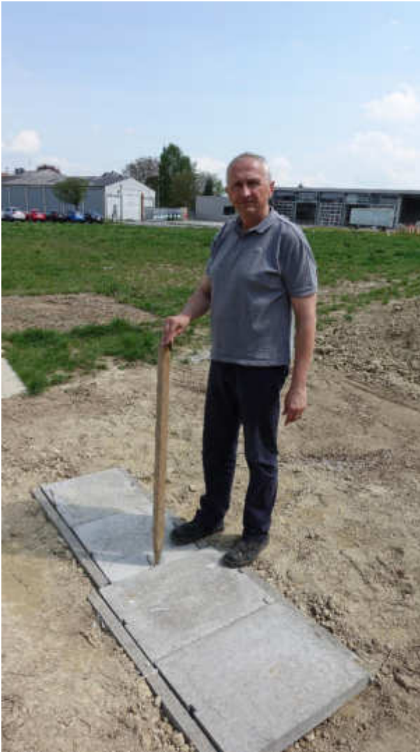
Abbildung 115: Drop tests with a bolt from a predefined height of 110 cm.
