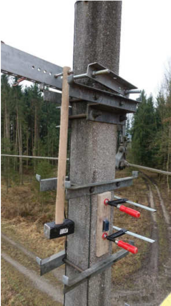
Abbildung 83: Sledgehammer and MSR-165 accelerometer mounted to the mast.
