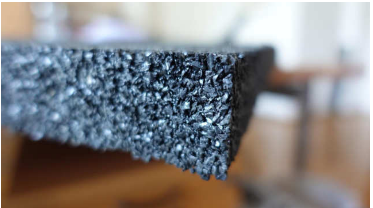
Abbildung 98: The troughs sit on these granule mats. Their specifications are 3 cm height x 20 cm width x 72.5 cm length for S4 troughs and 3 cm height x 20 cm width x 59.5 cm length for S3.
