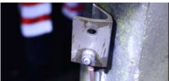
Abbildung 25: Experimental setup: Bracket and copper cable mounted to the foot of the mast.
